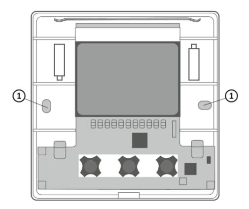
1. Holes for fixing screws.
