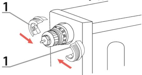
2. Tighten all the way the reduction fitting A (2) on the installed reduction fitting B (1)
