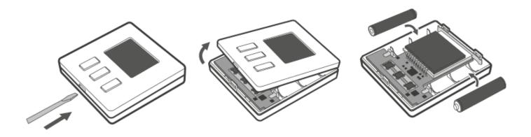
Place two AAA 1.5 V batteries in the battery socket observing the correct polarity.
