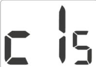
After correct installation on batteries, the LCD will display, for a second, all segments (display test) followed by the firmware version number. After a moment, the current temperature will be displayed. The controller is ready to use.
