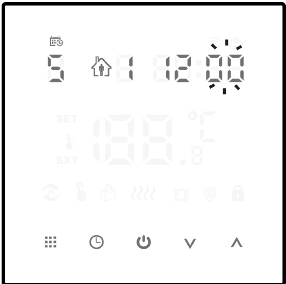
Use the (▼▲) buttons to select the program start minute, and then go to setting the temperature by pressing the (■) button.
