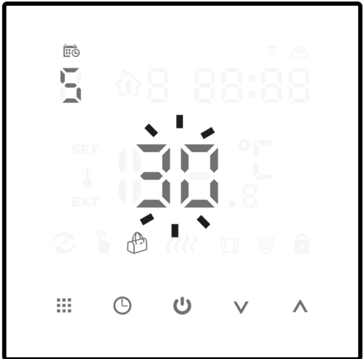
4. Then, use the (▼▲) buttons to set the desired temperature.
