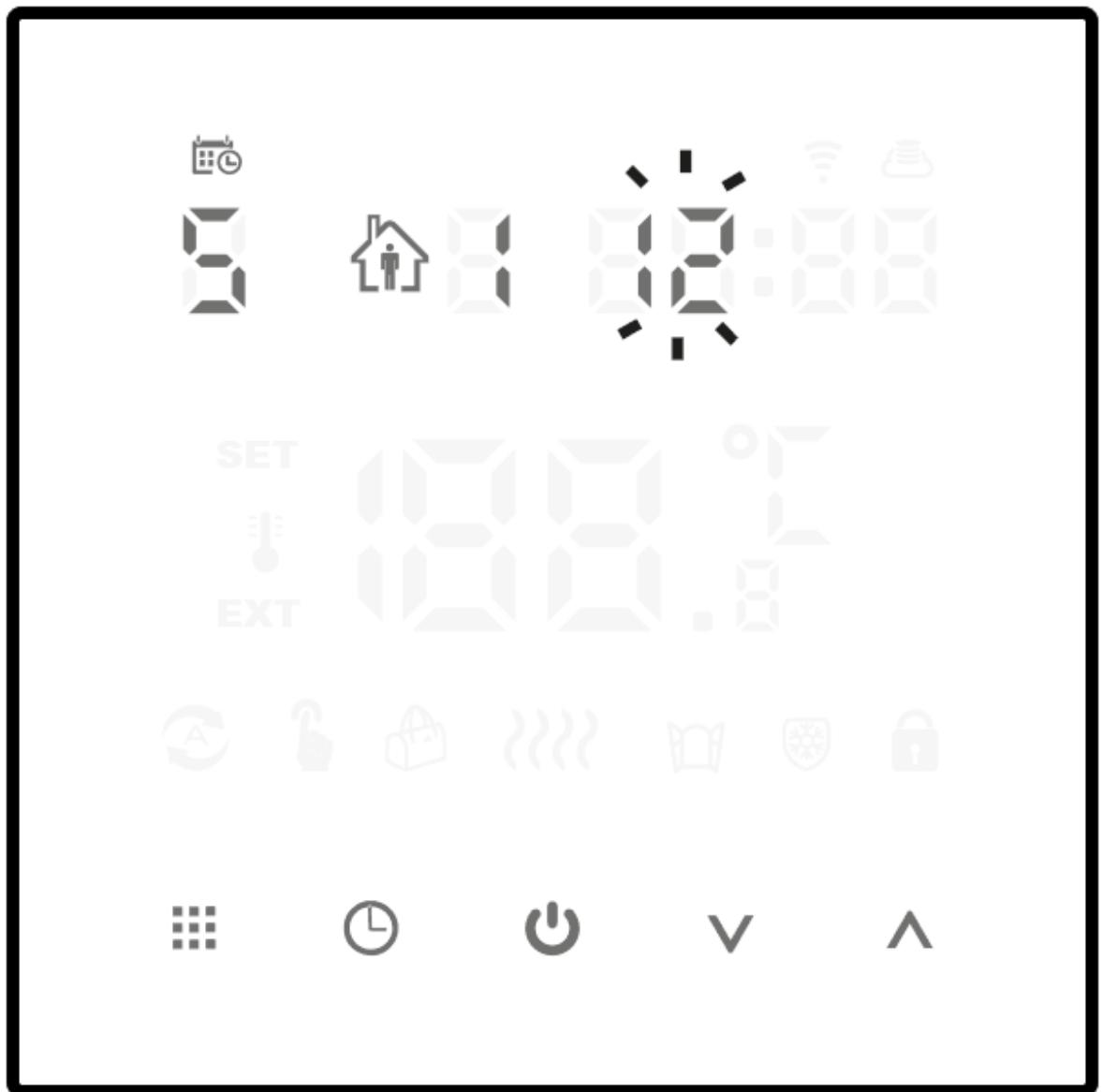
Use the (▼▲) buttons to select the program start hour, and then go to setting the start minute by pressing the (■) button again.
