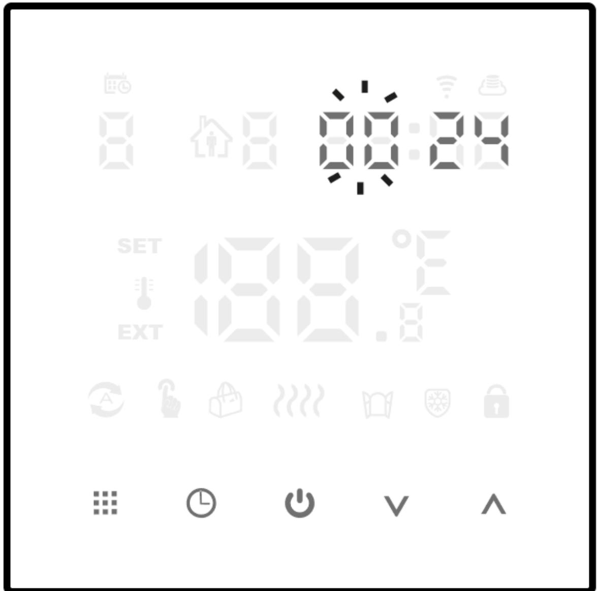
4. A flashing day of the week symbol will appear in the upper left corner of the display. Use the function buttons (**V****A**) to set the desired day of the week and confirm your choice with the (**O**) button.
