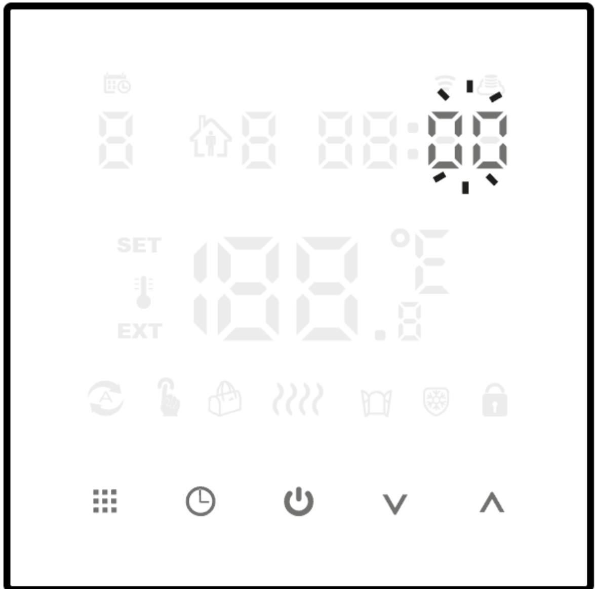
2. Use the function buttons (**V****A**) to set the desired minute and confirm with the (**O**) button.
