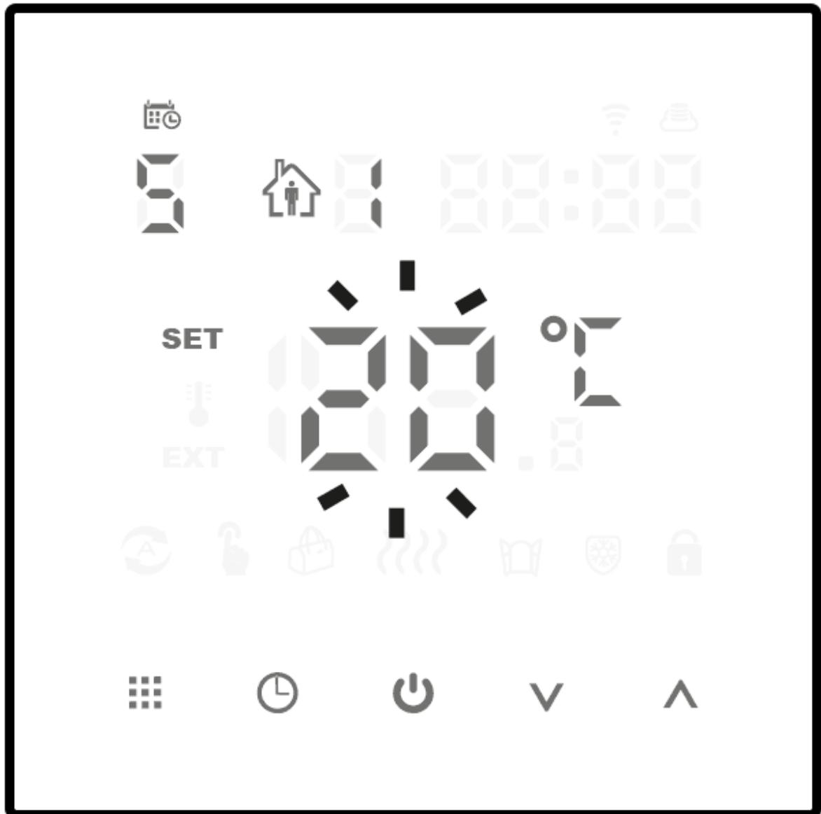
Use the (▼▲) buttons to select the program temperature, and then go to setting the next program by pressing the (■) button.
