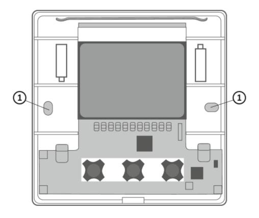
1. Holes for fixing screws.
