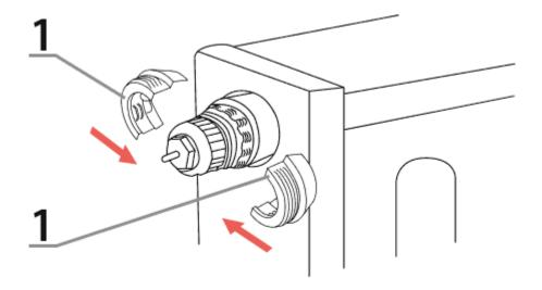
2. Screw face bushing B (2) onto the folded face bushing B (1) to the stop
