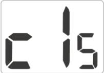
When the batteries are properly inserted in the sockets, the LCD display will show all segments for a second (display test) followed by the software version number. After a moment, the current temperature is displayed. AURATON Apus R is ready for operation.
