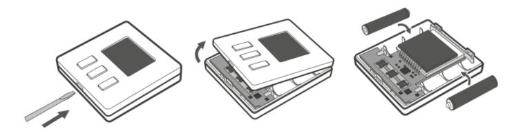
Insert two AAA 1.5V batteries into the battery socket, making sure that the battery terminals are properly aligned.
