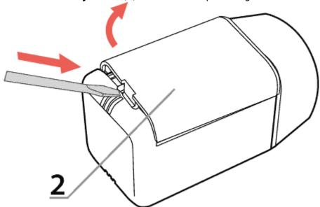
3. Install two AAA batteries in AURATON Apus paying attention to polarity. The head pin will move to the extreme open position, making it easy to mount the AURATON Apus on the face bushing.
