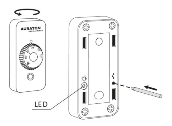
Pairing the AURATON Aquila Mini R (transmitter) with the AURATON Fornax is initiated by pressing the right pairing button () - a single beep on the AURATON Fornax receiver and holding it for at least 3 seconds until the LED starts flashing green (double beep), then release the button.
