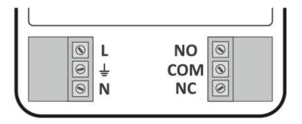
Connect the power supply wires to the clips of the power supply connector of the AURATON Fornax
