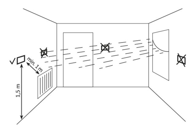
The correct operation of AURATON Aquila R is largely influenced by its location. Using the device in a
