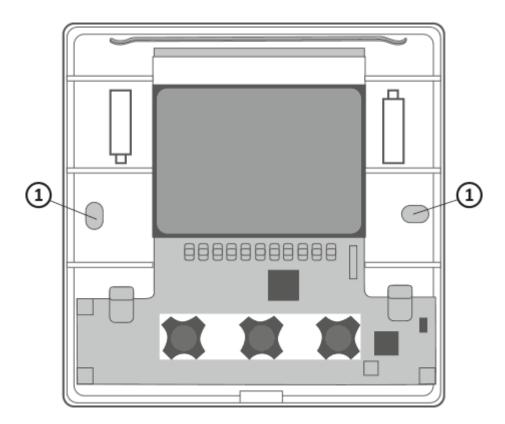
1. Holes for fixing screws.
