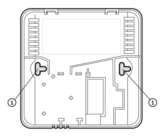
1 - Holes for fixing screws
