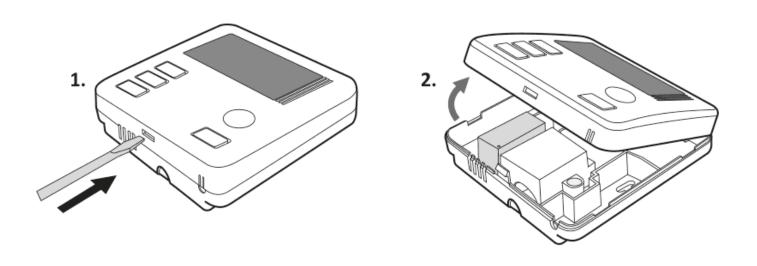
Wire terminals are located on the rear panel of AURATON Auriga, under the plastic cover.
