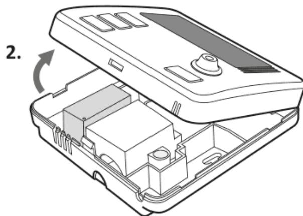
Wire terminals are located on the rear panel of AURATON Cetus, **under a plastic cover**.
