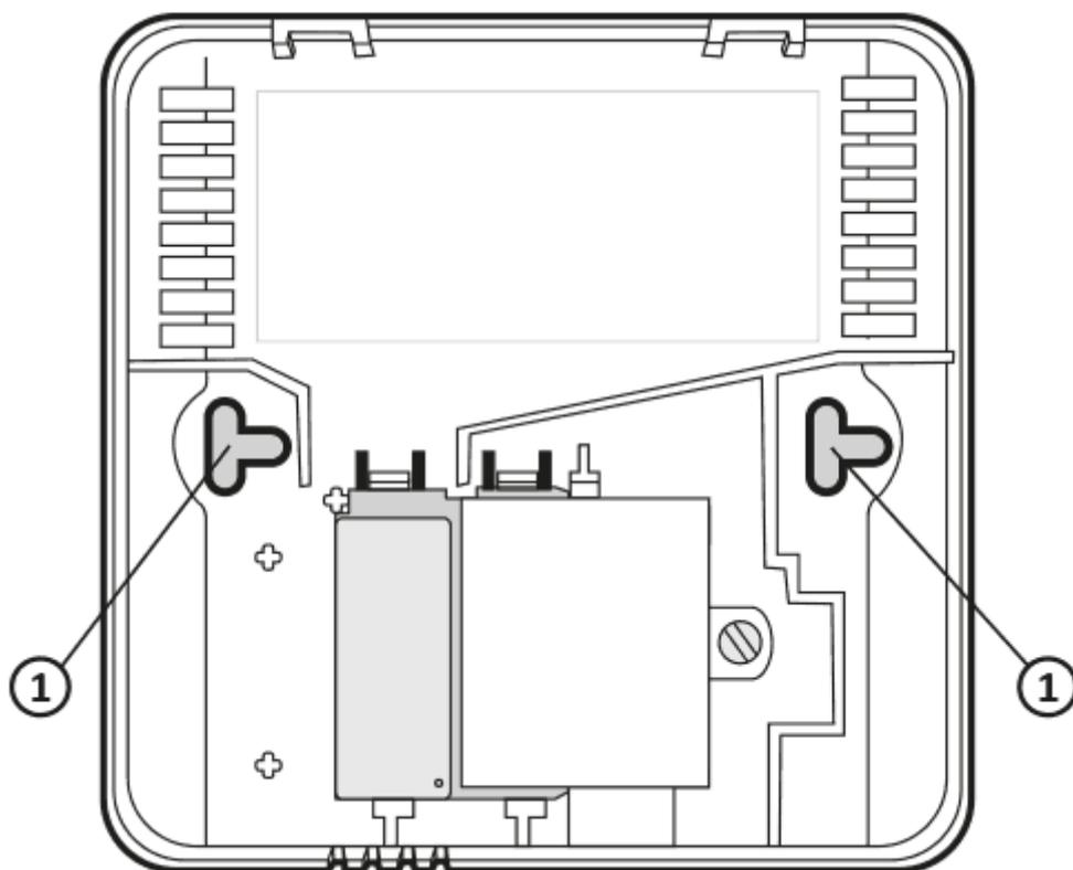
1. hole for fixing screw
