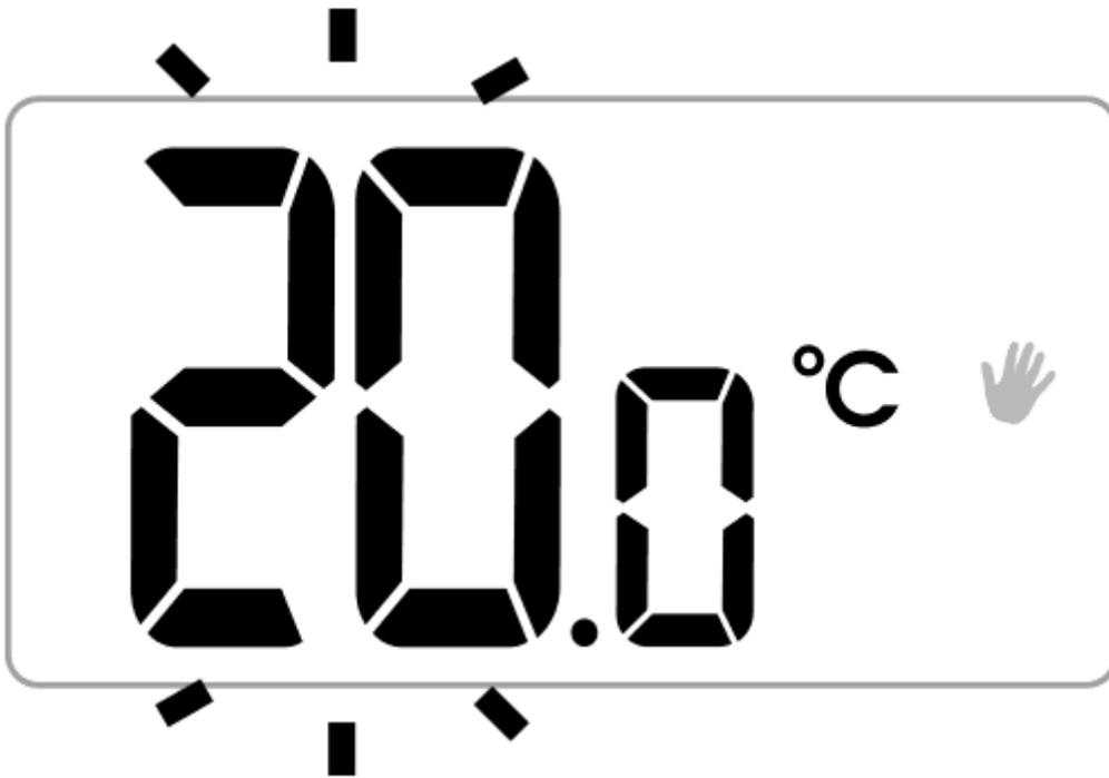
2. Turning the knob to the left or right sets the desired temperature value. Confirm the selection with
