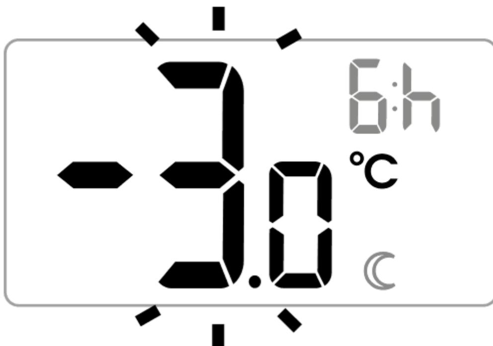
2. Turn the knob to the left or right to set the temperature lowering by 1 °C to 5 °C. Confirm the selection with
