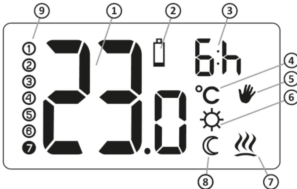
1. **Temperature** – In normal operation mode, AURATON Cetus displays the temperature of the room in which it is installed.
