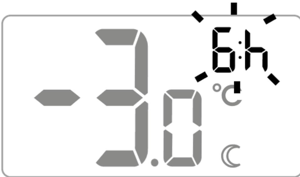
3. The hour field on the display will go into edit mode, and will start flashing. Using the knob again, set the number of hours for which the programmed lowered temperature is to remain valid. You can choose from 1 to 12 hours. Confirm the selection with
