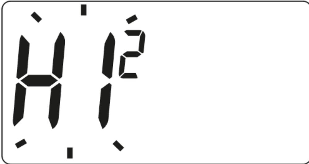
The hysteresis change mode is signalled by flashing HI. Turn the knob to the left or right to set the desired hysteresis.
