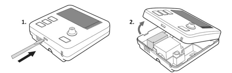
The terminals are located on the back of AURATON Libra, under the plastic casing.
