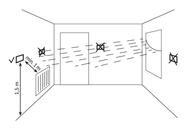
The correct operation of AURATON Libra is largely influenced by its location. Using the device in a place with no air circulation or a place with direct sunlight may result in incorrect temperature control. AURATON Libra should be installed on the internal wall of a building (a partition wall), in an environment with free air circulation. You should avoid proximity to heat-emitting devices (TV, heaters, refrigerators) or locations exposed to direct sunlight. The vicinity of doors and exposing
