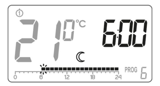
By pressing the 🔤 key and selecting time interval the entire program is modified.
