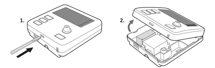
The terminals are located on the back of AURATON Libra H, under the plastic casing.
