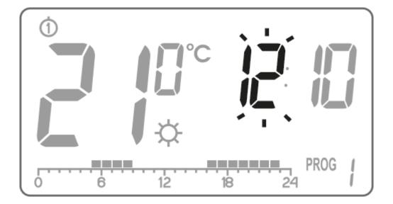
Turn the knob to the left or right to set the required hour and confirm with using the or button.
