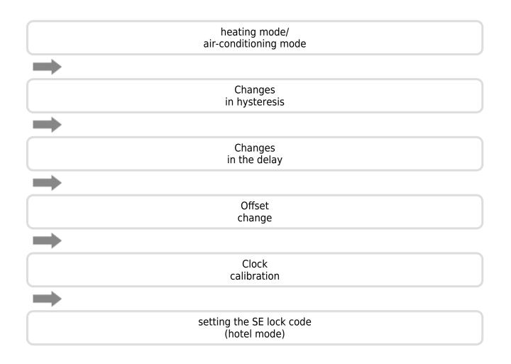
To enter the edit mode of the configuration settings, hold the **Proof** and **or** buttons simultaneously for 3 seconds until the settings menu is displayed.
