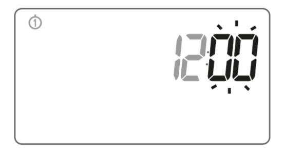
A flashing symbol of the day of the week appears in the upper left corner. Turn the knob to the left or right to set the day and confirm the selection using the  $\overline{o}$  button.
