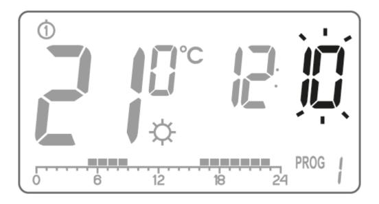
A flashing symbol of the day of the week appears in the upper left corner. Turn the knob to the left or right to set the day and confirm the selection using the or button.
