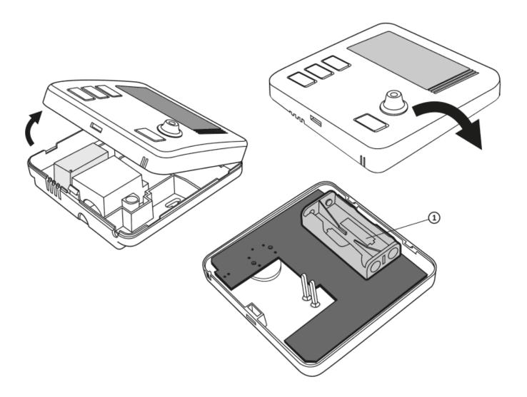
Insert two 1.5 V AAA batteries into the battery compartment, paying attention to the correct polarity of the batteries.
