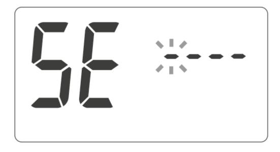
If you change the value from 0 to 9 using the +/- knob, press the  $\bigcirc$ . button within 10 seconds. Otherwise AURATON Libra H will leave this mode (normal operation) and the setting procedure will have to be restarted.
