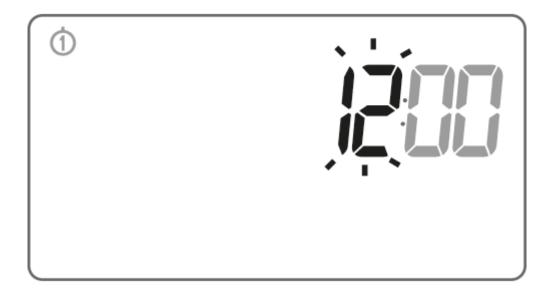
Turn the knob to the left or right to set the correct value on the minute segment and confirm using the ok button.
