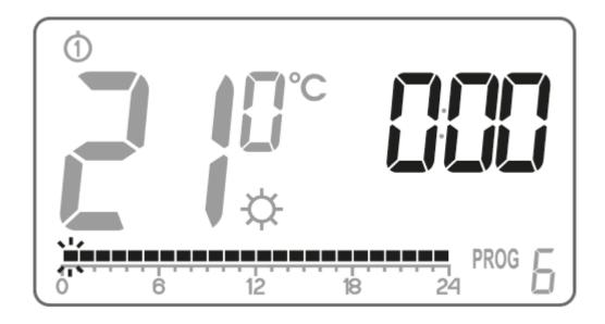
Press the key to select day (rectangle on) or night temperature (no rectangle). Then, select the time interval for the temperature selected with the knob.
