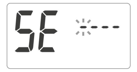
Use the +/- knob to set the code, press or after each digit is set (within 10 seconds of setting), otherwise AURATON Libra H will return to normal operation (lock on). After the correct code is entered, AURATON Libra H starts normal operation (lock off).
