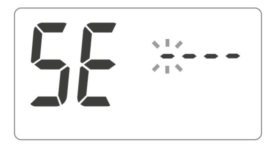
If you change the value from 0 to 9 using the +/- knob, press the or. button within 10 seconds.
