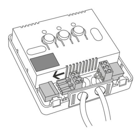
Connect the heating or air-conditioning device to the clips of the AURATON Fornax control connector. Follow the service manual of the heating or air-conditioning device. COM (common) and NO (normally open circuit) clips are most commonly used.
