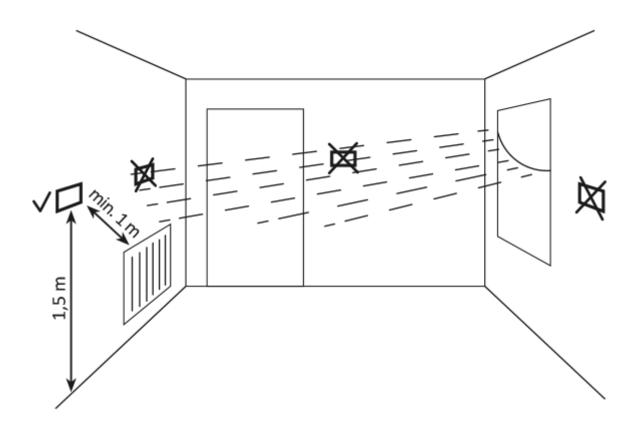
The correct operation of AURATON Libra RH is largely influenced by its location. Using the device in a place with no air circulation or a place with direct sunlight may result in incorrect temperature control. AURATON Libra RH should be installed on the internal wall of a building (a partition wall), in an environment with free air circulation. You should avoid proximity to heat-emitting devices (TV,
