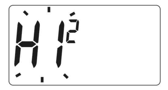
The hysteresis change mode is signaled by a flashing HI. Turn the knob to the left or right to set the desired hysteresis.
