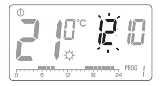
Turn the knob to the left or right to set the required hour and confirm with using the ox button.
