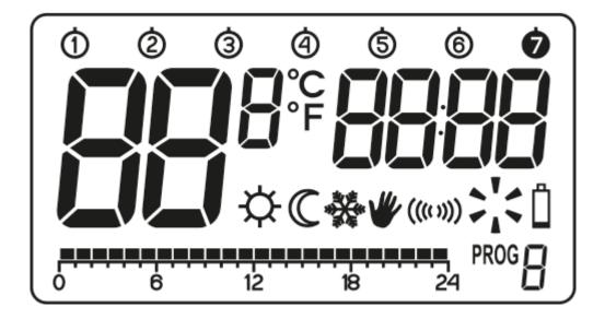
After a while, AURATON Libra RH will automatically switch to the time setting mode. A flashing item on the screen means that the device is currently in the edit mode. Turn the knob to the left or right to set the required hour and confirm using the ox button.
