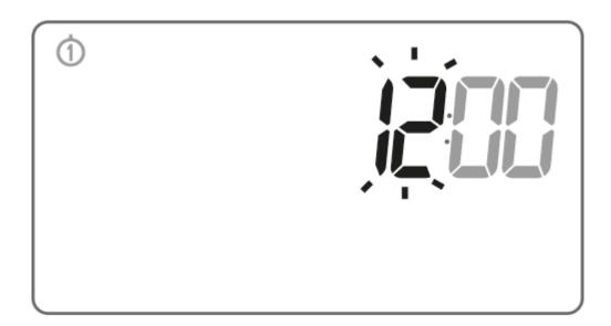
Turn the knob to the left or right to set the correct value on the minute segment and confirm using the ox button.
