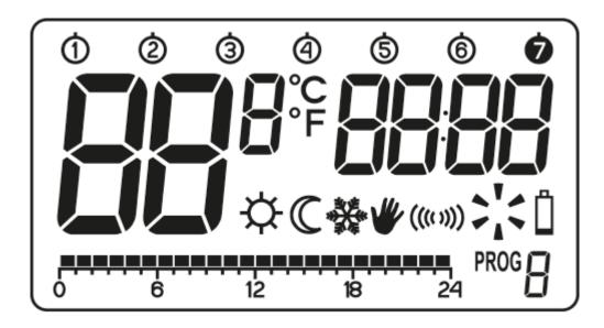
After a while, AURATON Libra R will automatically switch to the time setting mode. A flashing item on the screen means that the device is currently in the edit mode. Turn the knob to the left or right to set the required hour and confirm using the ox button.
