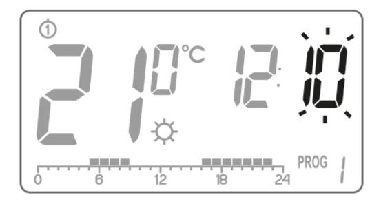
A flashing symbol of the day of the week appears in the upper left corner. Turn the knob to the left or right to set the day and confirm the selection using the ox button.
