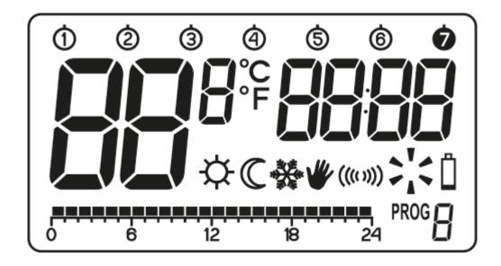
After a while, AURATON Pavo will automatically go to the hour setting. An item flashing on the screen indicates that it is currently in editing mode. Use the V buttons to set the desired hour and confirm the setting with the W button.
