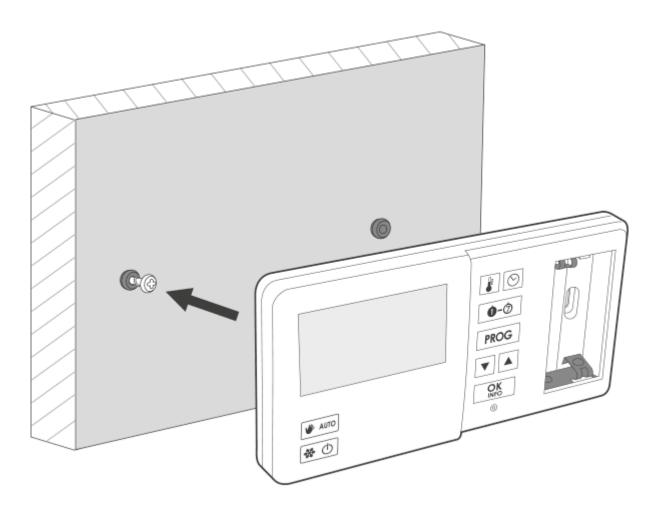
5. Tighten up the right screw so that it holds AURATON Pavo mounted securely.
