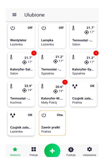
1. A red marker indicates update is available for the respective device. To download the update click and hold down respective icon for a while to move to the control screen.
