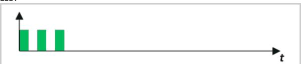
6. **Status:** Software upload failed, incorrect version in the memory or memory communication issue (3 blinks).
