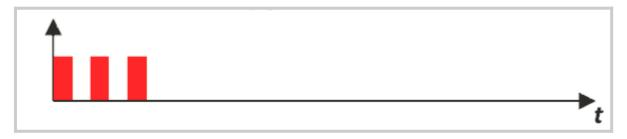
7. **Status:** Unexpected error during a software change that prevents proper device start-up. Service contact required.
