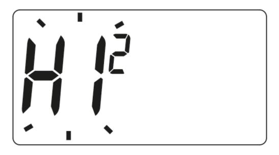
The hysteresis change mode is signaled by a flashing **HI**. Use the **V** buttons to set the desired hysteresis.
