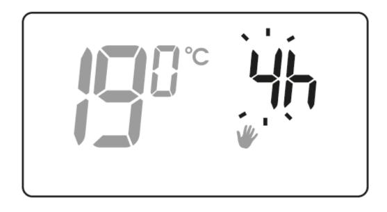
3. The temperature field starts flashing. It can be set with the **I** buttons. Confirm the selection with the **I** button.
