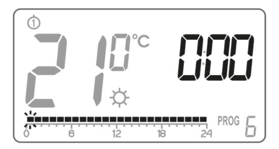
Press the  $\bigcirc$  or button to select the day temperature (a lit rectangle) or the night temperature (no rectangle) on the timeline.
