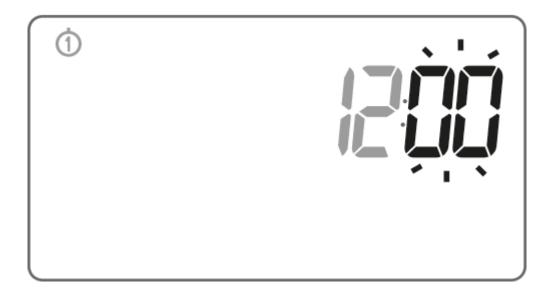
A flashing day of the week symbol appears in the upper left corner. Use the **I** buttons to set the desired day and confirm the selection with the **I** button. AURATON Tucana will enter its normal operating mode.
