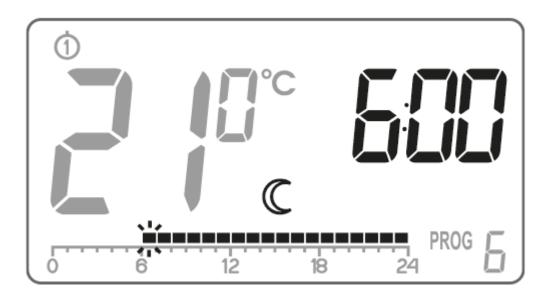
Use the **V** buttons to highlight subsequent hours on the timeline and select the day or night temperature for each hour (we toggle between a lit rectangle and no rectangle with the **C** button.
