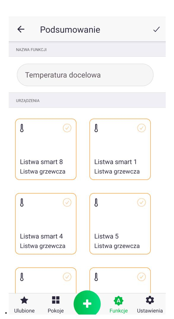
In order for the system to function properly, the current temperatures of the corresponding Smart series controller must be grouped with the current temperatures of the AURATON Floor Heating Controller. Proceed in the same way with the target temperatures if you want to control them from the front panel of the controller
