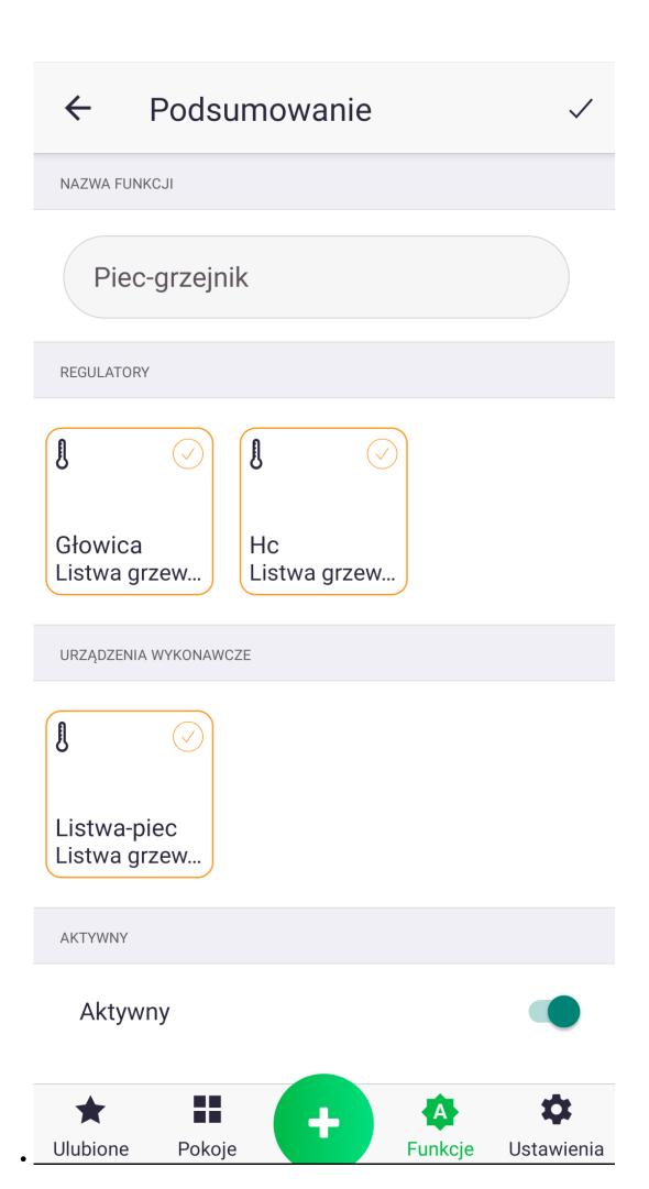
In order for the furnace (or furnace and pump) output to be activated not only when any of the AURATON Floor Heating Controller heating zones are active, but also when the thermostatic head (AURATON Radiator Controller) on the radiator initiates heating. To do this, add the "Heating" function, select the appropriate thermostatic head channel in the Controllers tab, and set the AURATON Floor Heating Controller furnace (or furnace and pump) channel as the actuator.
