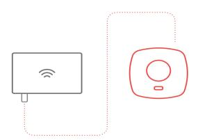
2. Use the MicroUSB-USB cable to connect Auraton Pulse with the power supply adapter. Insert the power supply adapter into the socket to power the central unit. After some time, the LED on the central unit should light up green to indicate the readiness for work.
