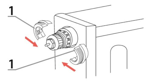
2. Screw tightly reduction A (2) onto the installed reduction B (1)
