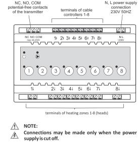
Each zone can be connected independently with one *AURATON* cable controller (e.g. A2025, A2030, A3003, and A3013).
