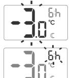
3. The hour field on the display will go into the edit mode and will start flashing. Use the knob again to set the number of hours during which the reduced temperature will be on. You can set from 1 to 12 hours.
