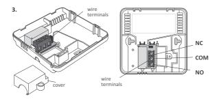
It is a typical bistable relay. The NC terminal is not used in most cases.
